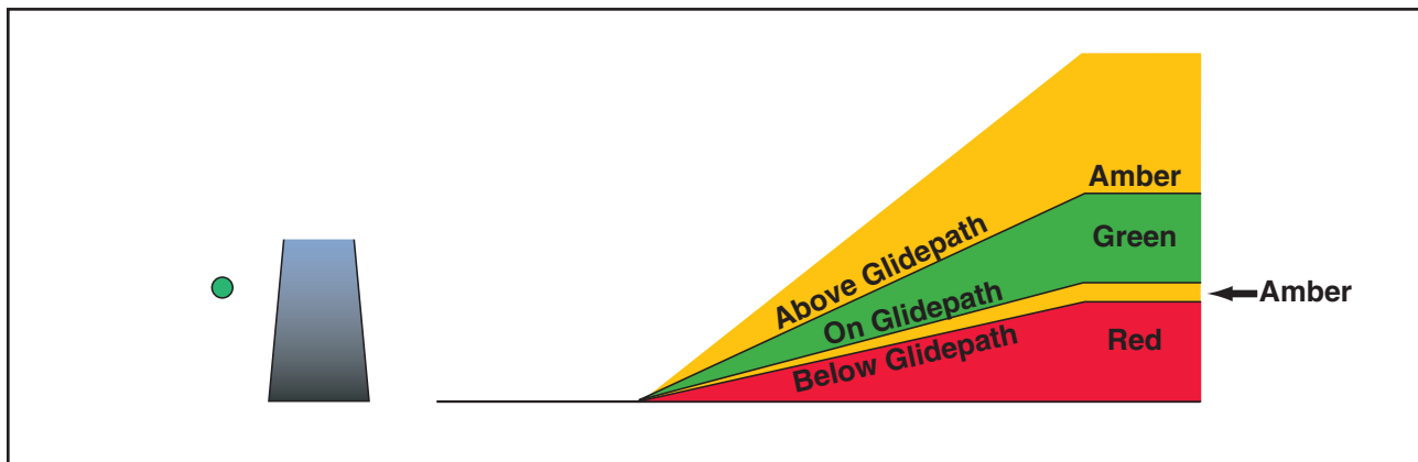
Figure 12-8. Tri-color visual approach slope indicator.
